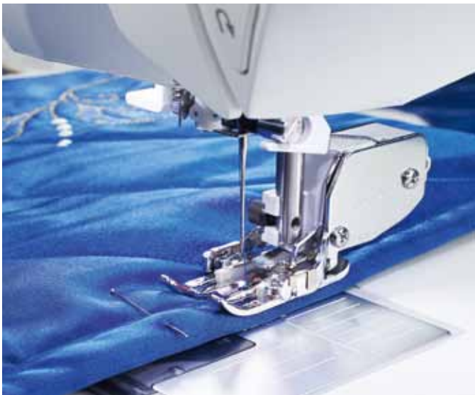
The Interchangeable Dual Feed is designed to feed layers of fabric and batting evenly, creating perfect feeding from the top and the bottom of your quilt.
