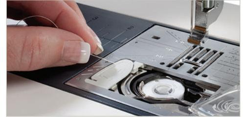
Slip the bobbin thread in the cover plate guide; the built in cutting blades trim the tail to the correct length for a super-clean start to your stitching line. After the initial threading, the auto-thread cutter takes care of trimming and re-setting the tails each time.
